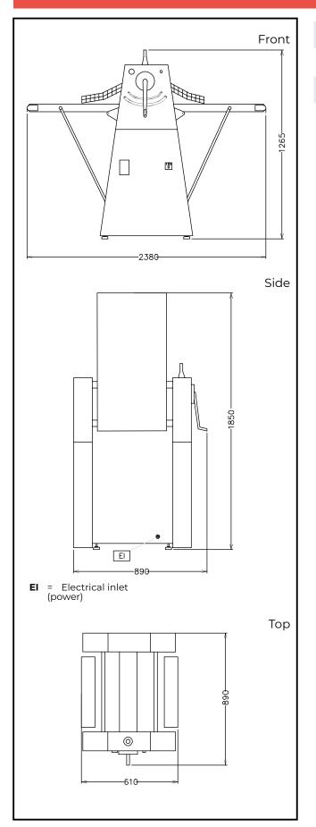
Electric Supply voltage: 230 V/1 ph/50/60 Hz 0.75 kW **Total Watts:** Key Information: External dimensions, Width: 2380 mm External dimensions, Depth: 890 mm External dimensions, 1265 mm Height: Net weight (kg): 160
